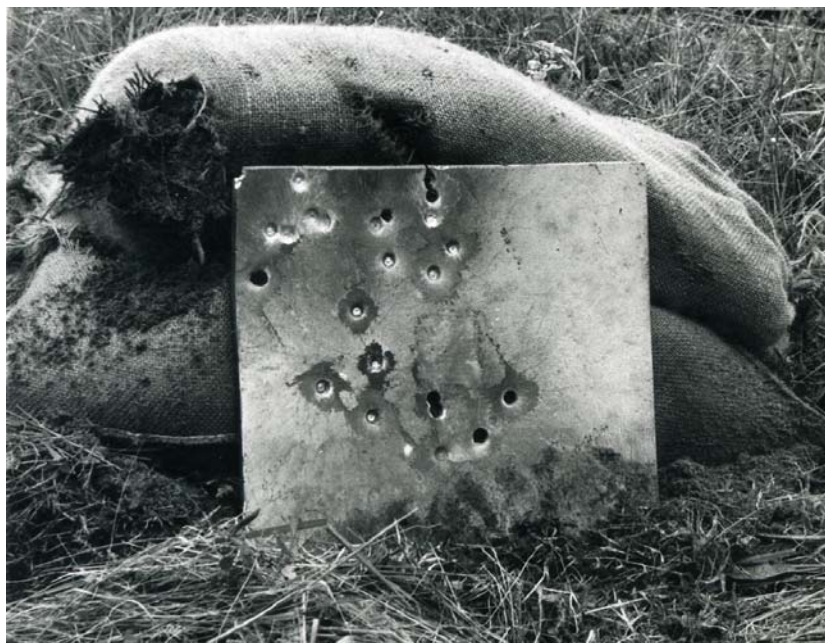
Plate of 363 Brinell Hardness as used on the Shorland Mark 1. Viewed from the front showing significant damage.
